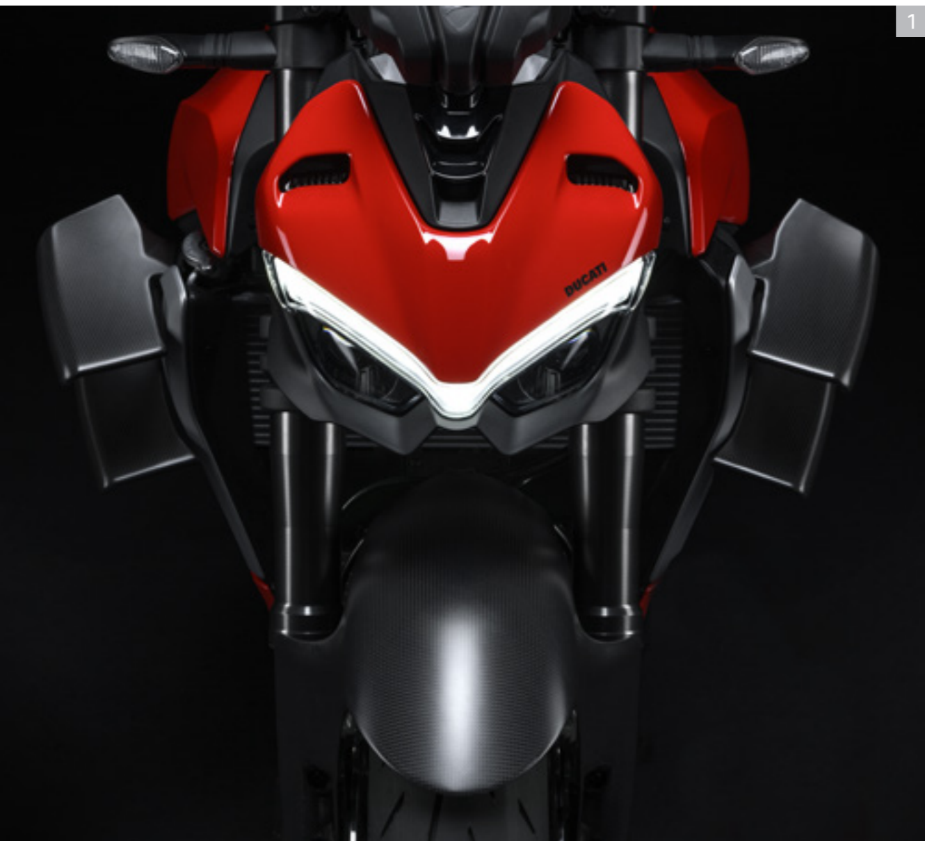
2 Carbon front mudguard. Set of carbon wings.
