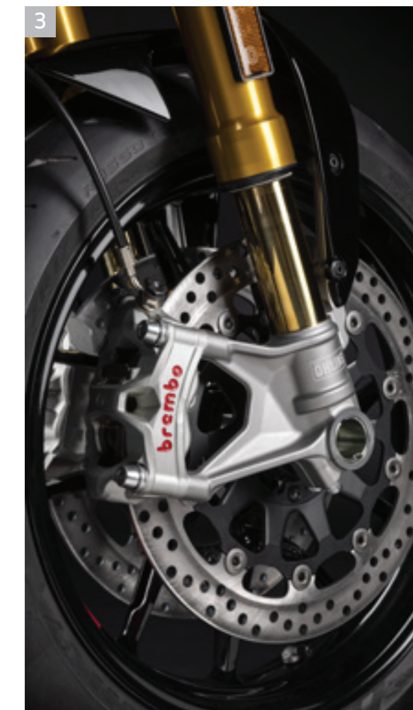
3 Radially mounted Brembo Stylema® monobloc 4-piston callipers
