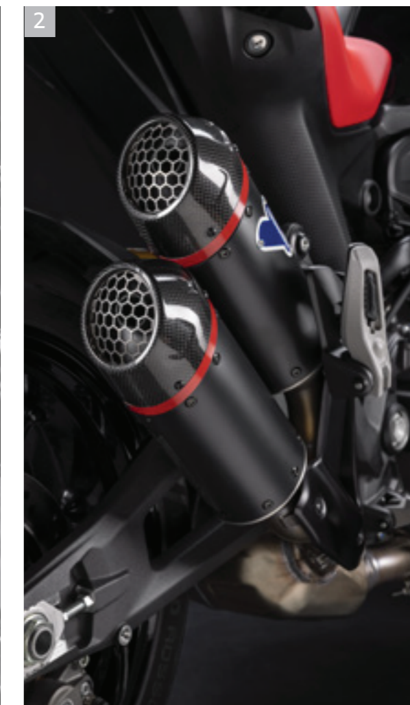
2 Pre-muffler and Termignoni type approved twin muffler, catalytic converter and 2 lambda probes
